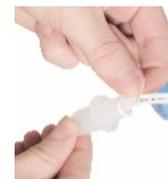
4. Guide the indicator strip into the sealing cap as far as possible.
